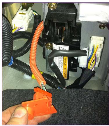
The connector to nowhere can be pulled out for better access.
