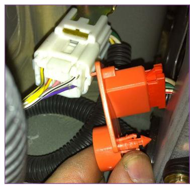
The connector holder is held in place with a push clip that can be removed using the service plug as a tool. One of the many clever ways the Toyota engineers try to keep us safe.
