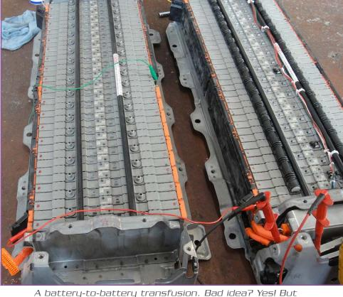
the HV battery is depleted. Other drivers may give up quickly, but then the tow driver tries a few times, and the car gets moved a few times in the shop, then by the time you're ready to diagnose the problem, there's only a crank or two left, or maybe none at all.
