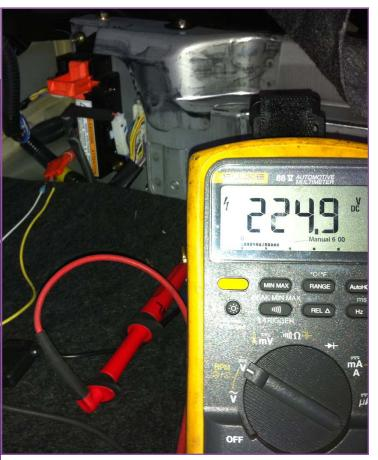
When the reading is positive, the meter is hooked up correctly. Don't make the connection with a live circuit! Disconnect the service plug before connecting your meter, then plug it back in to take the reading.
