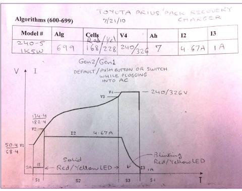
might damage the battery. To avoid this possibility, the charger defaults to the lower voltage. That way, there's less risk of an incompetent user damaging a battery pack. If a Gen1 is charged with the lower voltage, it won't be hurt, it just won't charge fully.
