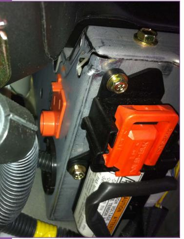
Once the cover has been pulled back, you'll be able to see the connector to nowhere and the interlock. ALWAYS remove the interlock before touching any orange (high voltage) components!
