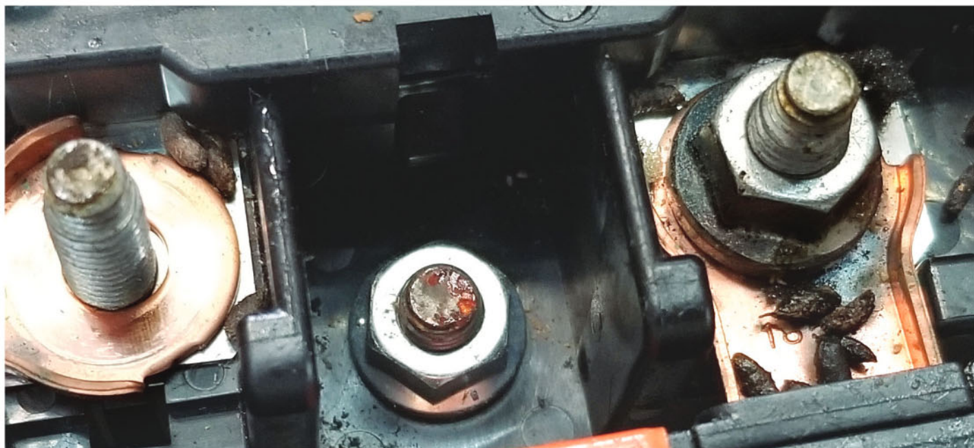
Mouse urine is conductive enough to cause a high voltage short to ground. This 2013 Prius required a major disassembly and cleanup to correct a P0AA6 (and a very foul odor).
