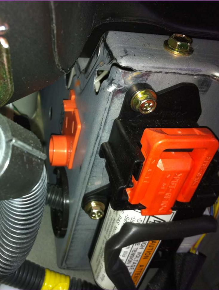
Once the cover has been pulled back, you'll be able to see the connector to nowhere and the interlock. ALWAYS remove the interlock before touching any orange (high voltage) components!
